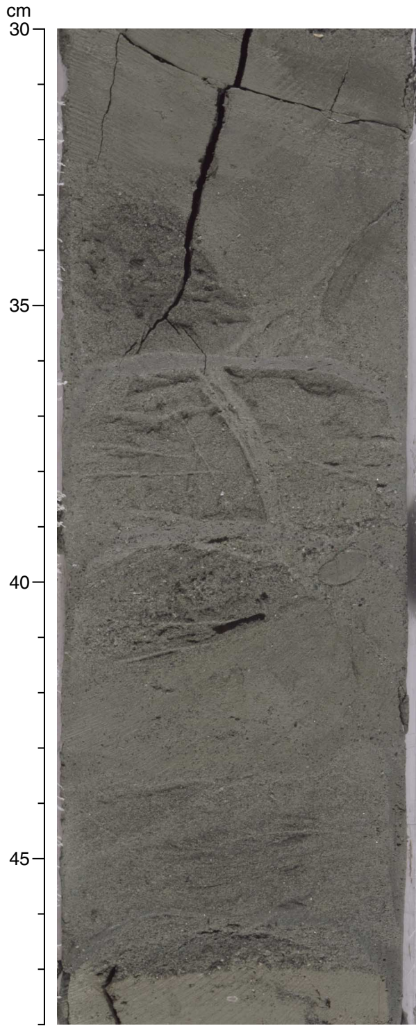
Figure F13. Poorly lithified coarse sand of Section 190-1175A-44X-1 (406.86 mbsf) exhibiting apparent web structure. Note, however, that the thick, convex-upward horizontal bands are interpreted as induced by XCB coring.
