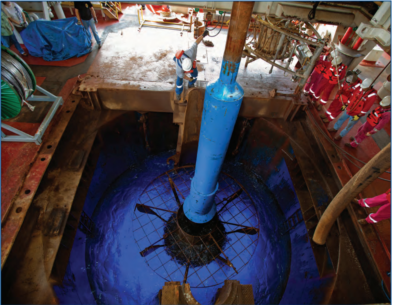
Pulling the Hole 395A CORK through the JOIDES Resolution moonpool
