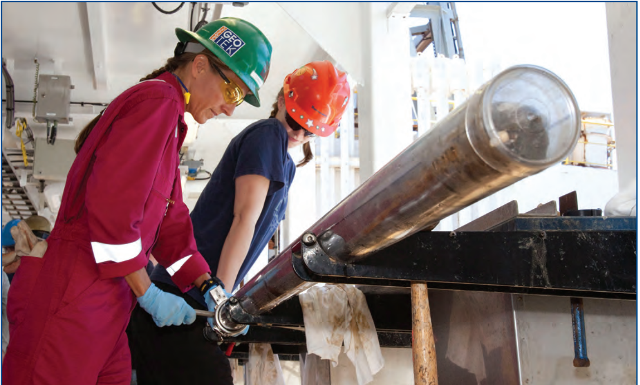
Cutting the core liner
