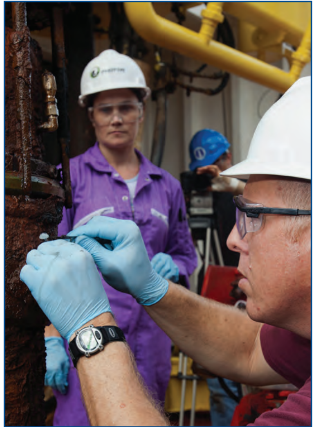
Scraping microbiological samples from the recovered Hole 395A CORK
