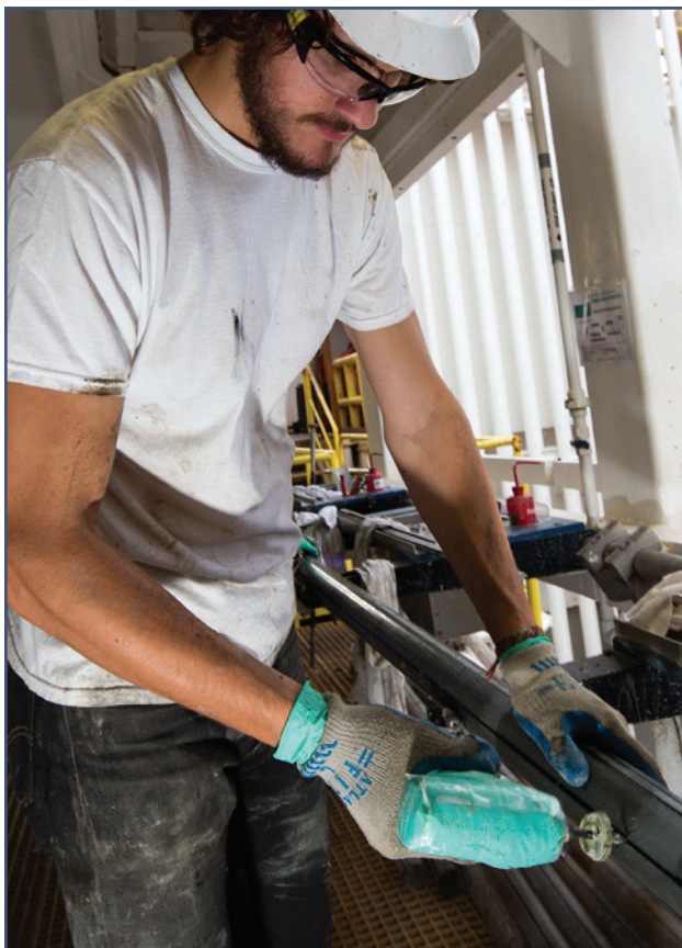
Drilling holes in the core liner to relieve gas pressure
