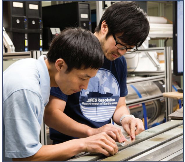
Scraping the core face in preparation for core imaging
