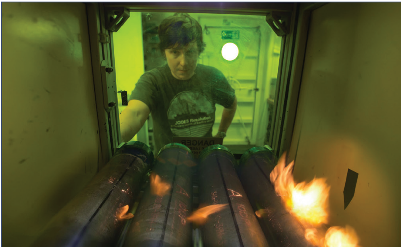
Monitoring the core-liner laser engraving process
