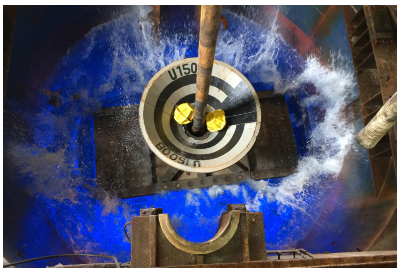
Reentry cone with mud skirt attached splashing into the moonpool.
