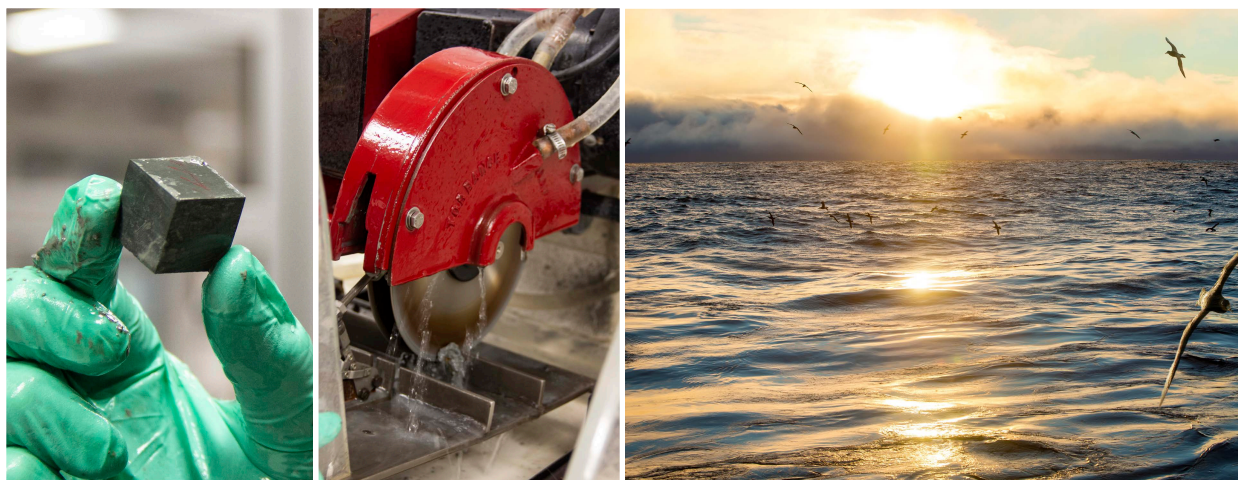
From left: Paleomagnetic cube sample. Using the rock saw to cut a paleomagnetic cube sample from mudstone. Sunrise from the JOIDES Resolution .
