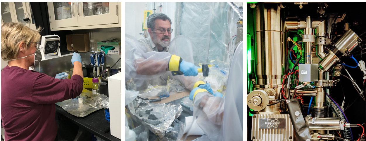
From left: Working at the KOACH clean bench. Collecting microbiology rock samples in the glove box. New scanning electron microscope with electron dispersive spectrometer for deployment on the JOIDES Resolution .
